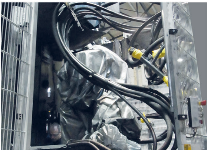
Spray robot to the forge for cooling and spraying of separating agent
