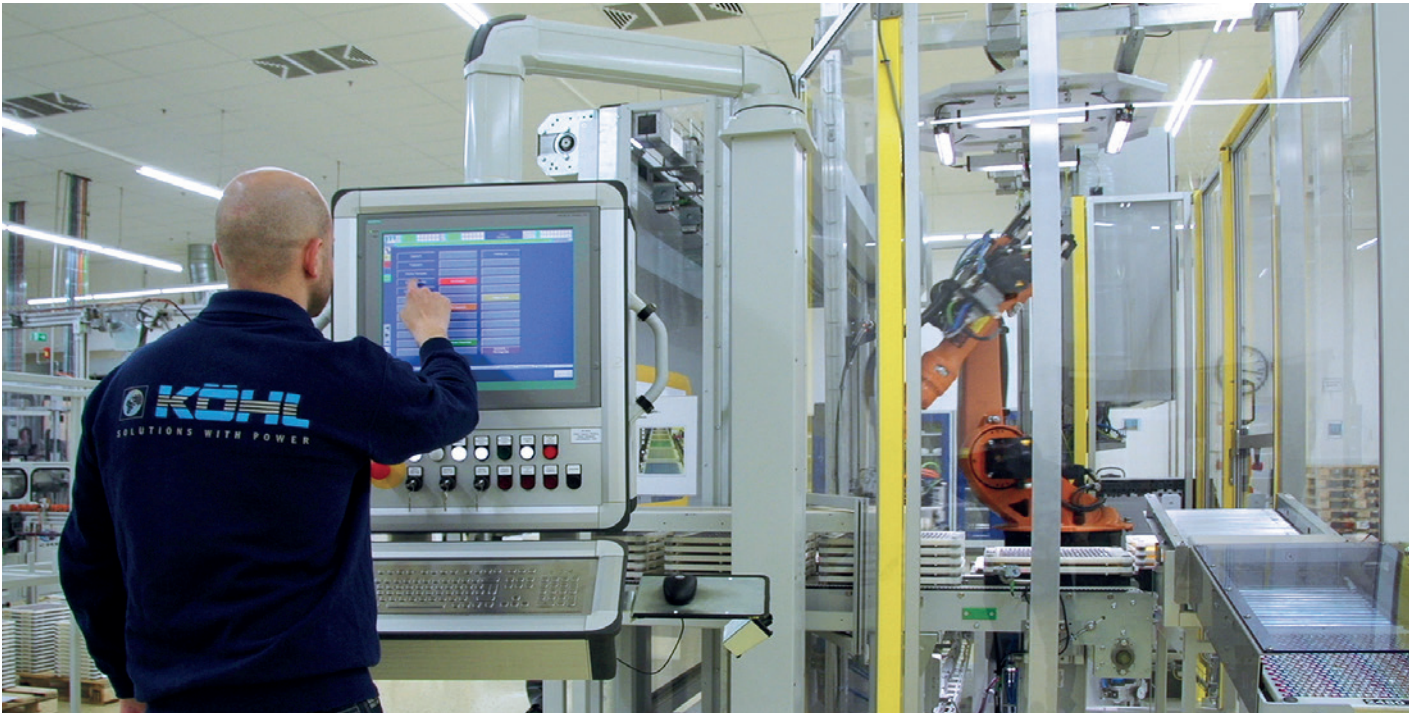
Operating a mobile robot cell for picking aroma capsules
