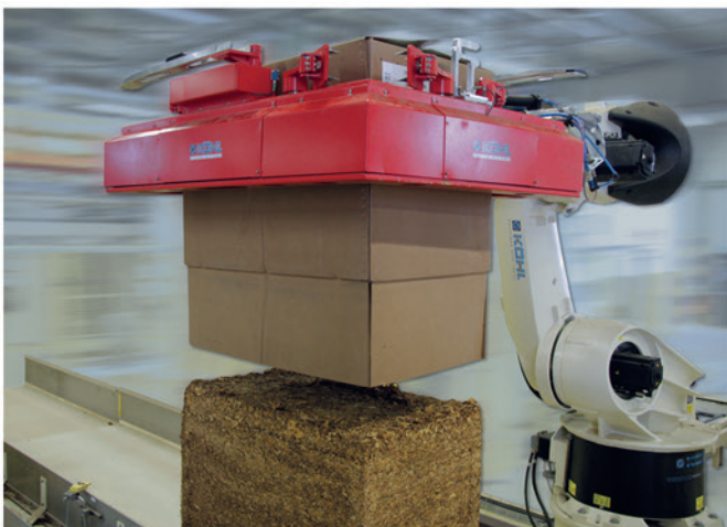
Patented unpacking-gripper for raw tobacco
