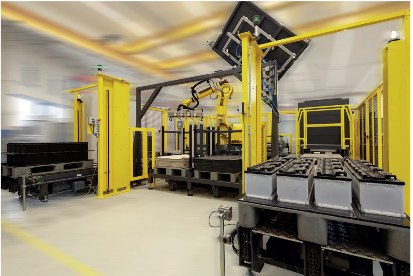
Fully-automatic robot cell for the palletization of different ready-to-be-dispatched car batteries
