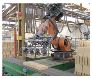
The KÖHL focus of the handling and automation systems for the refractory industry lies on completely automated systems for kiln car loading and removal of the formed products from the press. Industrial robots from the leading manufacturers, such as e.g. ABB, FANUC and KUKA or, if needed, also portals will be used, depending on the requirement and customer wishes.
