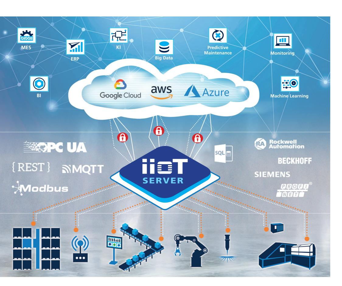
The KÖHL IIoT-Server is a smart Machine-To-Cloud solution that collects and handles data at the shopfloor level and forwards it to a Cloud or Fog environment.
