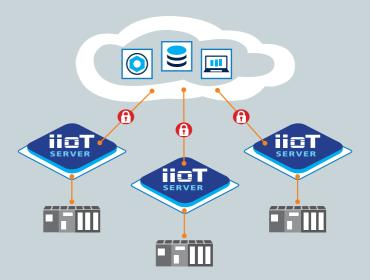
Each PLC is connected to a separate unit of the KÖHL IIoT Servers. The minimal hardware requirements allow the use of cost-effective and space-saving control cabinet solutions. The data can be transferred from the production network to the cloud in a secure way.
