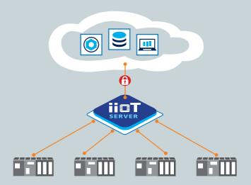
All PLCs of a production line or an entire plant are connected to a central unit of the **KÖHL IIoT Servers**. This can be easily integrated into existing server or virtualisation architectures.
