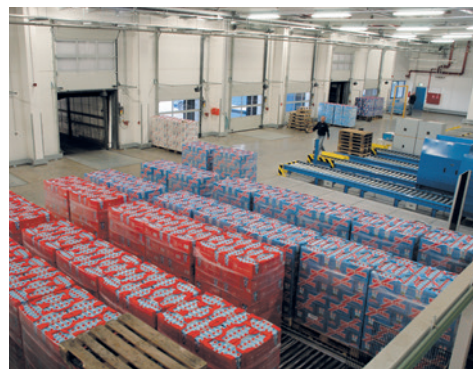
Individual goods ready for delivery, shown as a flow storage with separation mechanics at the appropriate end of the lane.
