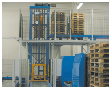
Vertical conveyor and empty pallet checking station.
