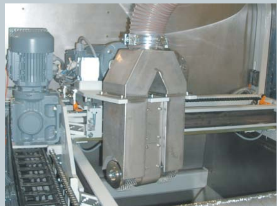
Cleaning carriage: Rotating twin-brushes clean the scraping belt from the collected foreign bodies.
