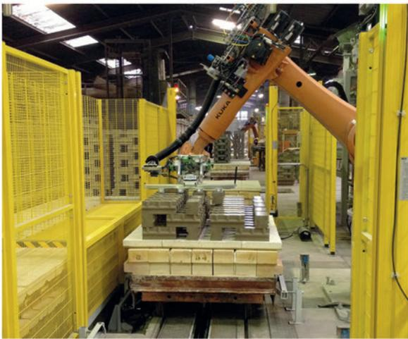
The KÖHL focus of the handling and automation systems for the refractory industry lies on completely automated systems for kiln car loading and removal of the formed products from the press. Industrial robots from the leading manufacturers, such as e.g. ABB, FANUC and KUKA or, if needed, also portals will be used, depending on the requirement and customer wishes.
